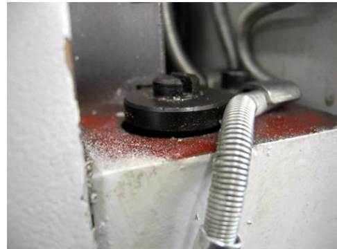
Figure 9.1a – Upper Z gib screw
