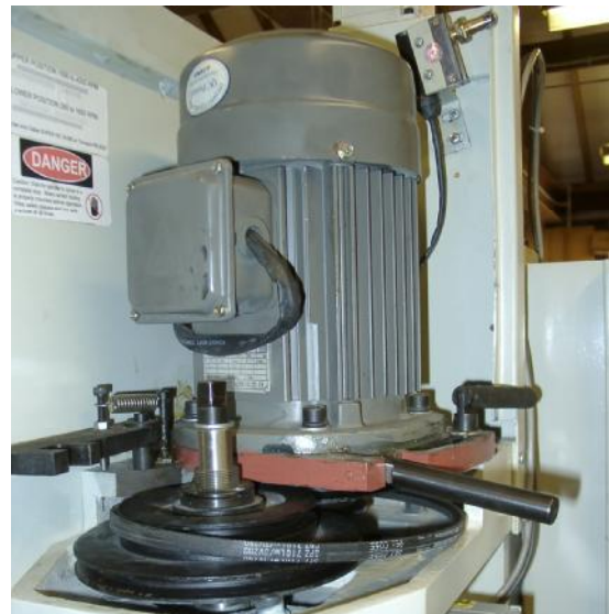
Figure 5.8 – Changing spindle speed range
