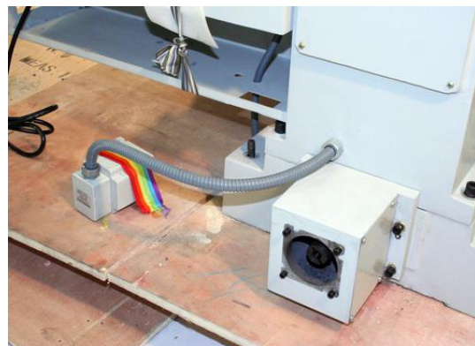
Figure 2.5 – Y-axis motor as shipped and mounting flange
