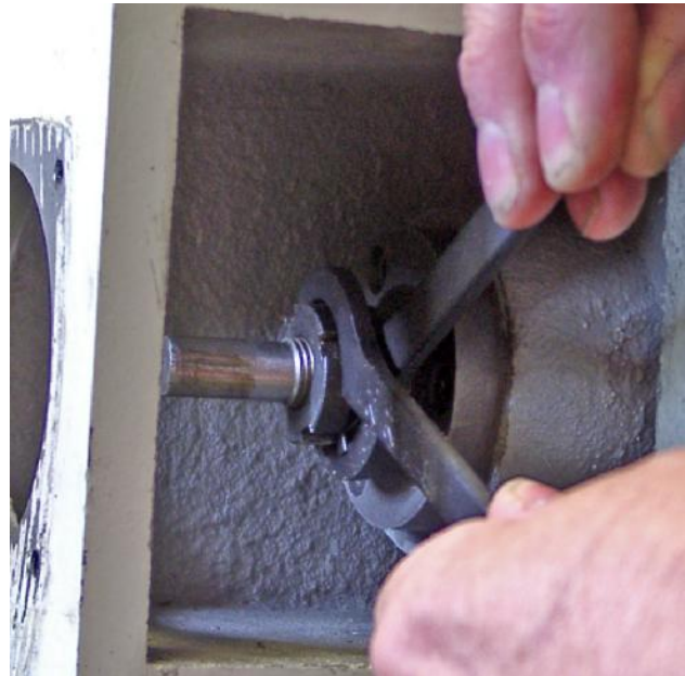
Figure 9.7 – Tightening the lock nut
