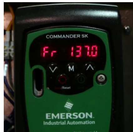
Figure 9.9 – VFD frequency readout Using Tormach PCNC 1100 Series II
