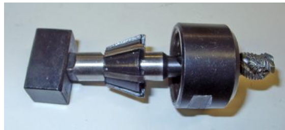
Figure 8.24 – Tap collet and anti-rotation block
