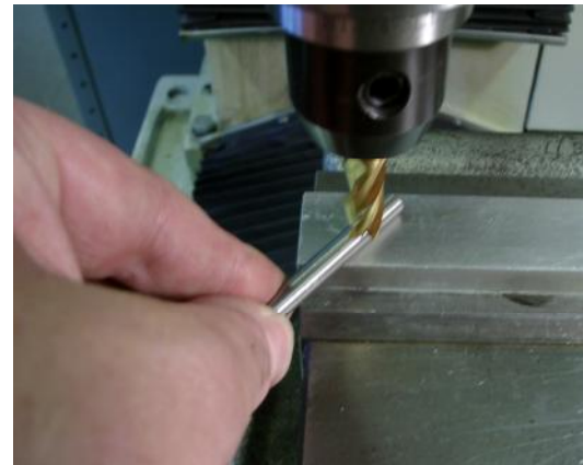
Figure 6.13 – Gauge just rolls under tool
