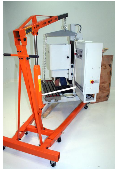
Figure 2.7 – Hoist bar for slinging the mill
