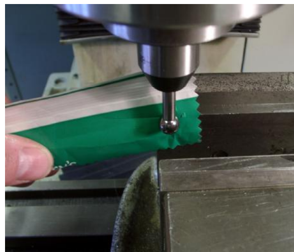
Figure 6.22 – Measuring vise jaw Y position
