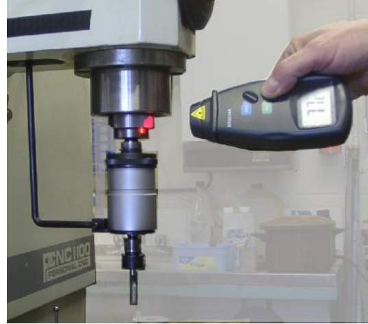
Figure 8.27 – Measuring spindle speed
