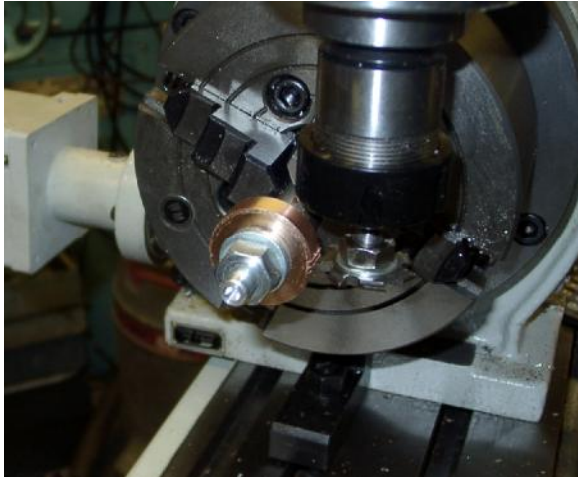
Figure 8.4 – Gear cutting (tailstock removed for clarity)
