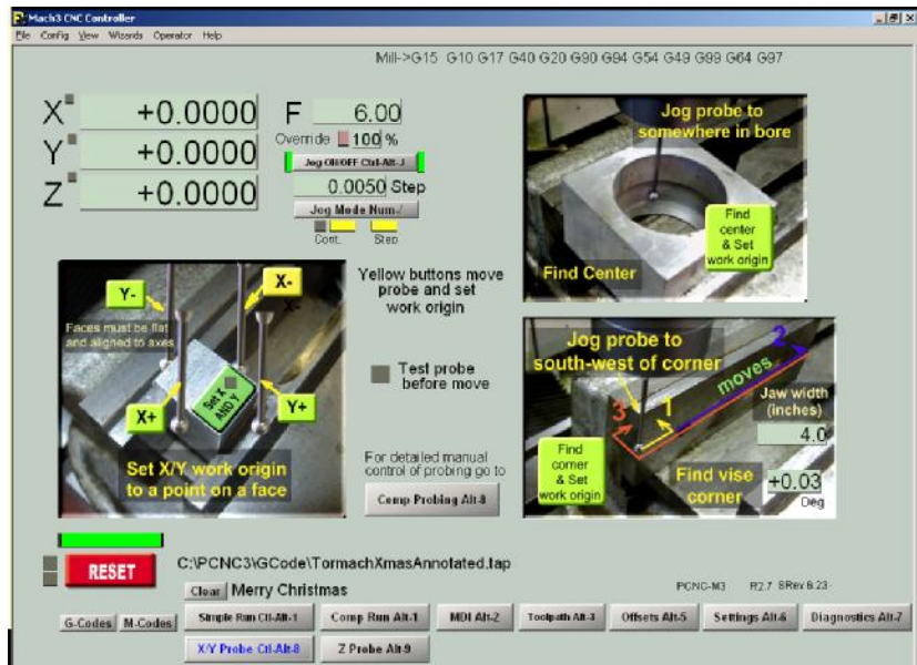
Figure 8.10 – Simple XY Probing
