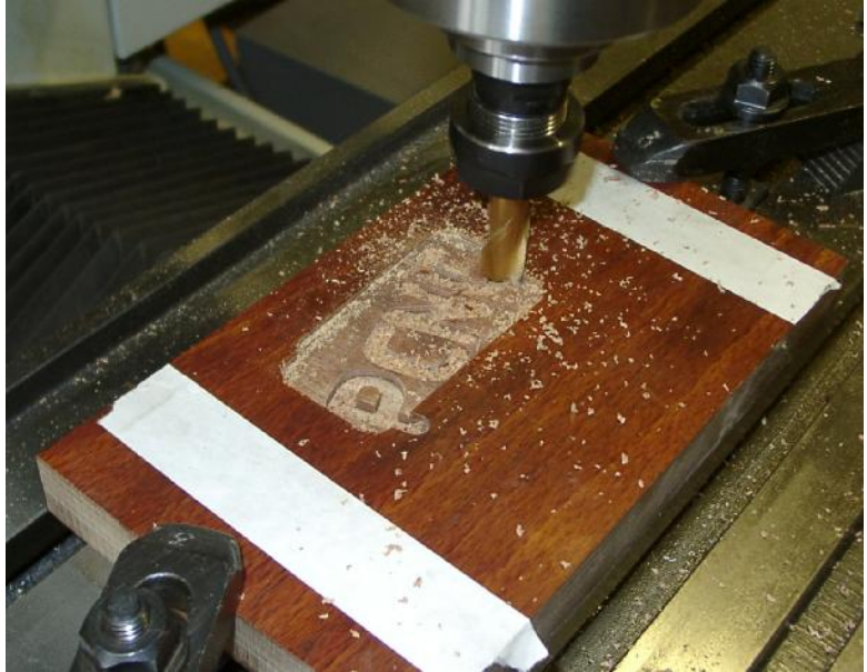
Figure 3.10 – Cutting the pocket
