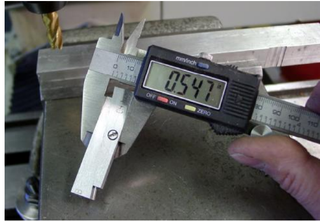
Figure 6.15 – Measuring the parallel gauge
