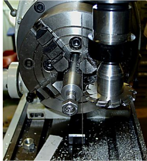
Figure 8.5– Ruler vertical so on center
