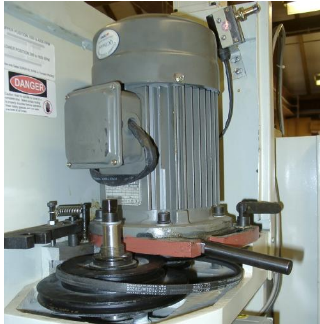
Figure 2.17 – Changing spindle pulleys
