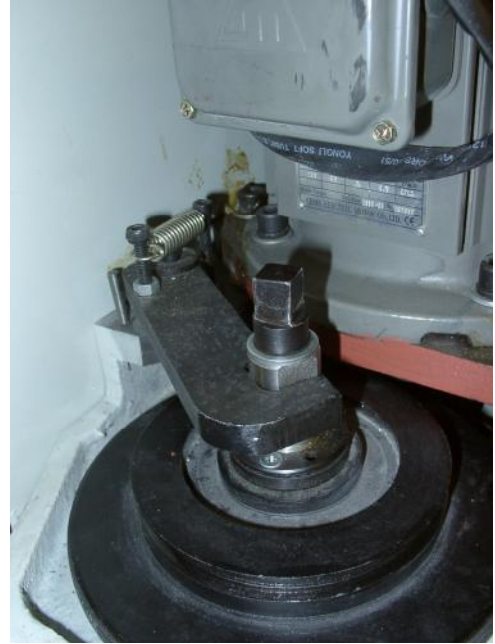
Figure 5.7 – Spindle lock fork engaged
