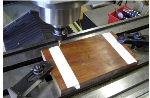
Figure 3.6 – Tool setup at zero points
