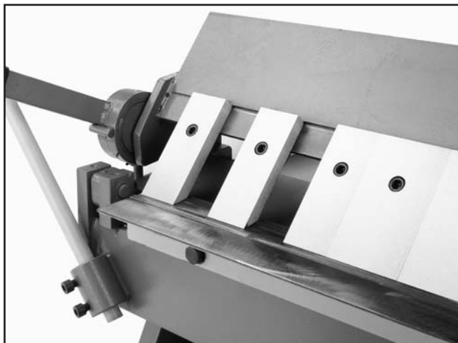
Figure 11. Fingers removed to provide space for matching fingers with box or pan widths.
